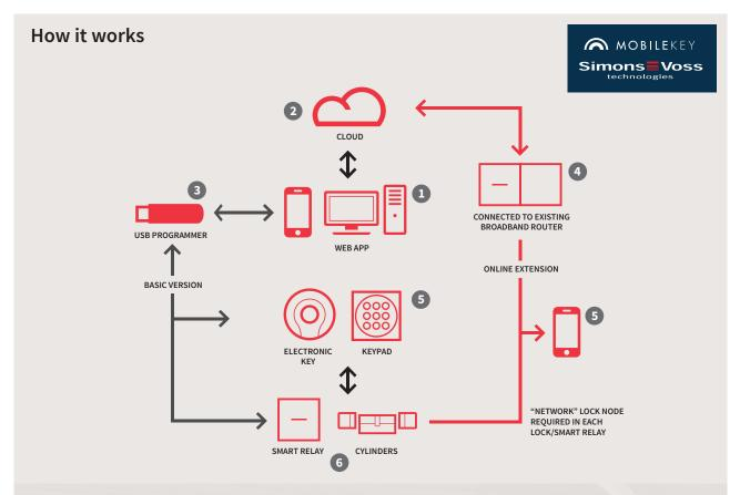
Easy to install, set up and manage, Mobile Key brings wireless access control to your small or medium-sized business. For up to 20 doors.
