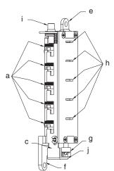
Position the chamber in one hand, as shown. Hold chamber by the top screw tab (e) and bottom screw tab (f).
