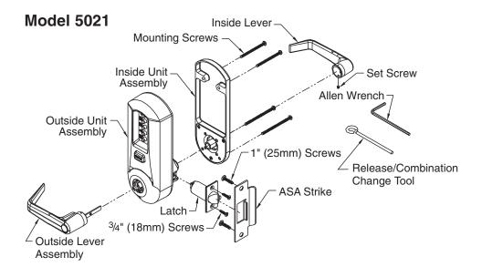
The Simplex 5000 (Model 5021 shown above) is a non-handed lock that is preassembled for left-hand installations. It is field reversible.
