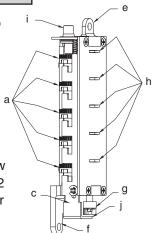
Push the shoulder (j) at the bottom of the Unlocking slide up toward the code change button and release. If each of the 5 "L" shaped legs of the unlocking slide engages snugly inside its corresponding code gear pocket, then it confirms that the new code has been successfully changed. Rotate the reset cam (g) back toward you and release.
