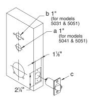
A-5 Secure the latch to the door using two ¾" (19 mm) combination screws (d) supplied. Latch unit faceplate must be flush with door (e).
