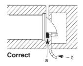
N-2 Mark locations where the gaps are approximately %6" (5 mm). Make sure these locations are free from grease and dust. Peel the bumpers (c) (supplied) from their protective backing without touching the adhesive surface and stick them on the marked locations.
