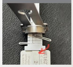
Attach the separate tension bar as shown and you can pick and decode the lock.
