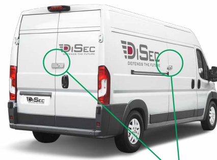
POSITION OF LOCKS ON REAR AND SIDE DOORS.
