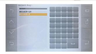
• **Step 2** Tap "Confirm", select the key type and then (1)tap "Key Decode" to decode your customer's key as shown below. (2) Alternatively, if you already know the height of the 9 bittings, simply enter them and proceed to cut the key. Follow the on-screen instructions to cut the key.
