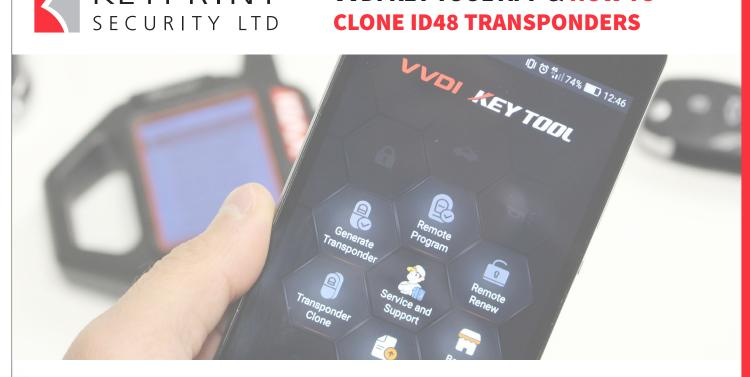
**Step 5** Put the blank ID48 transponder chip into the left coil of the Key Tool and press **Write** to write the date onto the new chip.
