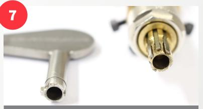
When the lock is open, tighten the nut wheel in the picked position to keep the arms in place. You can now use the tool as a trial key.
