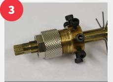
Adjust the nut wheel so that the picking arms can freely move.
