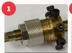
Loosen the nut wheel and the seven grub screws.
