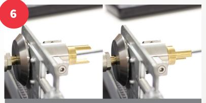
Continue the picking process on all the pins until the lock opens.
