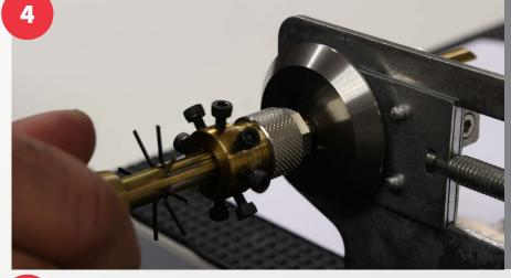
Insert the tool into the lock with the red dot adjacent to the vertical slot of the lock Then apply tension left or right. As with any picking process, tension control will determine the pins that are moving and those that are solid.
