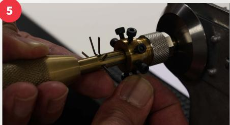
Use the arms to pick the solid pins. Once you have picked a pin and you can see a springy movement, tighten the grub screw to hold the <u>arm and pin in position.</u>
