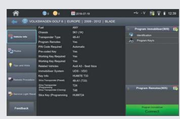
A simple grid provides all the information to identify the vehicle you want to program, including VIN number, transponder type, immo-
