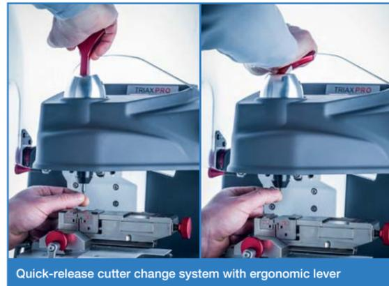
Quick-release cutter change system with ergonomic lever
